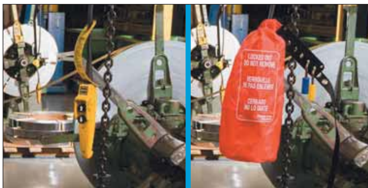
Hoist Control Lockout
